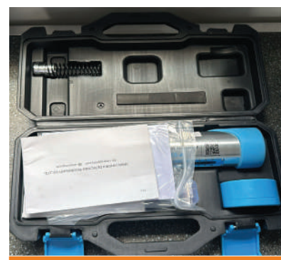
4.) Concrete Test Hammer (Schmidt Hammer) N type
